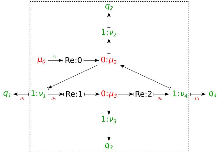
Figure 3: The bond graph representation of Michaelis-Menten open system with enzyme degradation.
